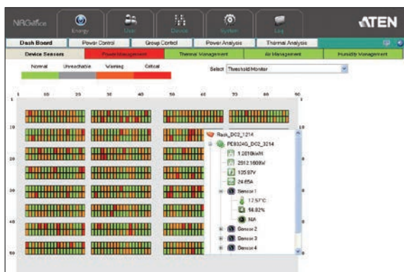
Real-time Rack Status Monitoring
